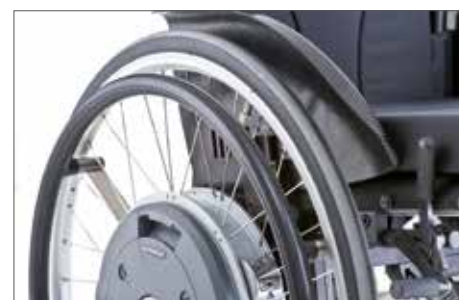
Rubber-coated push rims for improved grip
