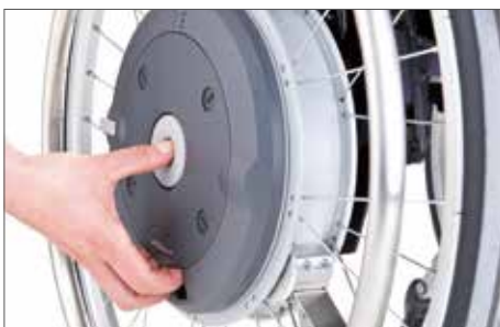
Removing the e-motion wheel from the wheelchair
